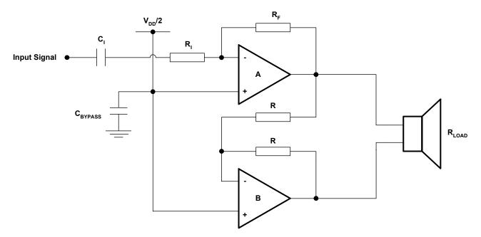
Figure 3. The BTL Audio Power Amplifier
