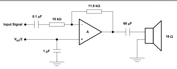
Figure 2. The SE Audio Power Amplifier Example
