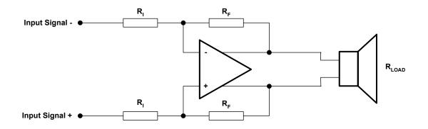
Figure 5. The Fully Differential Audio Power Amplifier
