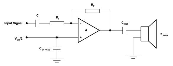
Figure 1. The SE Audio Power Amplifier
