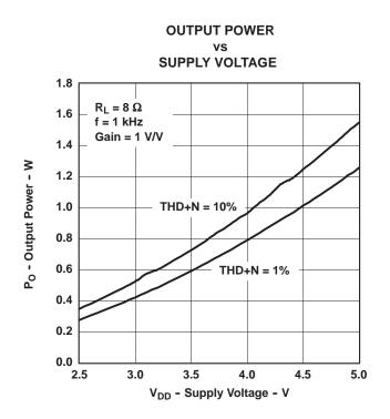
Figure 6. Output Power vs Supply Voltage Graphs for the TPA6203A1
